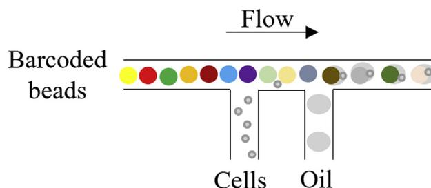
**Figure 5.** Microfluidics device for single-cell and barcoded bead encapsulation in oil emulsion.
